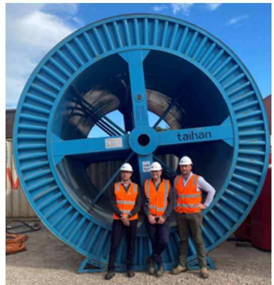
Our engineers Jonas, Jono and Will with a 4.5 m drum carrying 1000 m of cable
